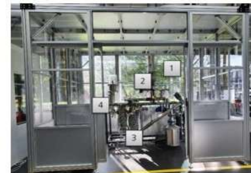
TCR®-2 plant and components: 1) Feed hopper, 2) Reactor, 3) Post-Reformer, 4) Condensation unit
